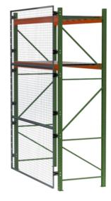
RACK GUARD PANELS CAN EXTEND OVER THE TOP OF THE UPRIGHTS UP TO 2' WITHOUT REQUIRING AN EXTENSION. IF OVER 2' A MAX OF 4' EXTENSION CLIPS ARE REQUIRED.
